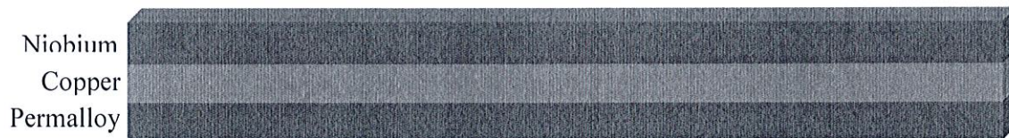
Figure 1: The tri-layer used within this study uses Permalloy as the ferromagnet as the source of spin pumping. The niobium is separated from the permalloy by a copper spacer intended to disrupt any proximity effects.
